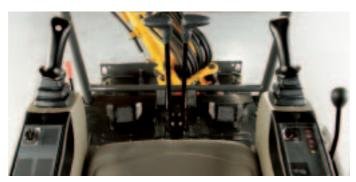
A user-friendly operating environment designed for long days of productive work and minimal operator fatigue: hand or foot operated travel controls, readily visible instrument panel, unrestricted visibility in all directions. Two travel speeds: 2.0/3.5 kph
