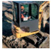
CX 18B fitted with an hydraulically adjustable track gauge (990 mm - 1300 mm) allows easy access through narrow openings or increases stability for heavy digging and lifting.
