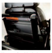
New comfortable vinyl leather-look, water resistant, adjustable suspended seat, with large document storage, wide tiltable and adjustable armrests and retracting seat belt.
