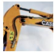
Standard auxiliary hydraulic functions (single or double acting) with piping/hoses up to the dipper and "ready to work" hydraulic Quick Hitch.
