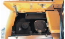
2 variable displacement axial piston hydraulic pumps feeding the attachment, the travel and the swing.
