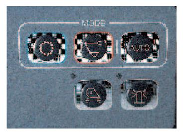
The **AUTO** mode on the new CX230 considerably simplifies machine operation, since it enables the working mode to be changed automatically and continuously (without any action on the part of the operator), depending on the type of work being done. Over all the cycles performed, a real reduction in fuel consumption is found compared with continuous use in one single working mode.
