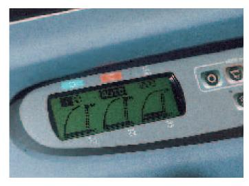
L mode (Light) is the mode to be used for finishing work (sloping banks, profiles, etc), where precision is required. It's also the mode used when handling loads and travelling with loads, due to the reduced flow and the continuous availability of Power Boost (maximum pressure applied continuously).
